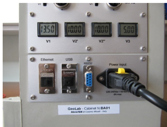
Fig. 16 - Detail of the main supply and connectivity options of the cabinet; digital voltmeters V1, V2', V2'' and V3 installed in order to monitor the various output voltages.
