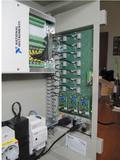
Fig. 15 - Internal view of one data acquisition cabinet based on a National Instruments' USB DAQ device
