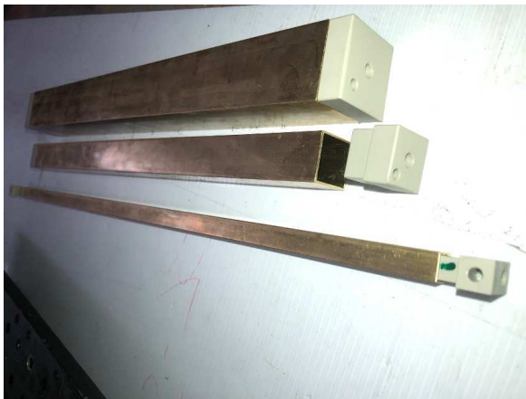
Figure 7.2: Left: set of drift tubes with different cell sizes used in the beam tests. Right: portable gas system used for gas-flow monitoring and gas mixing.
