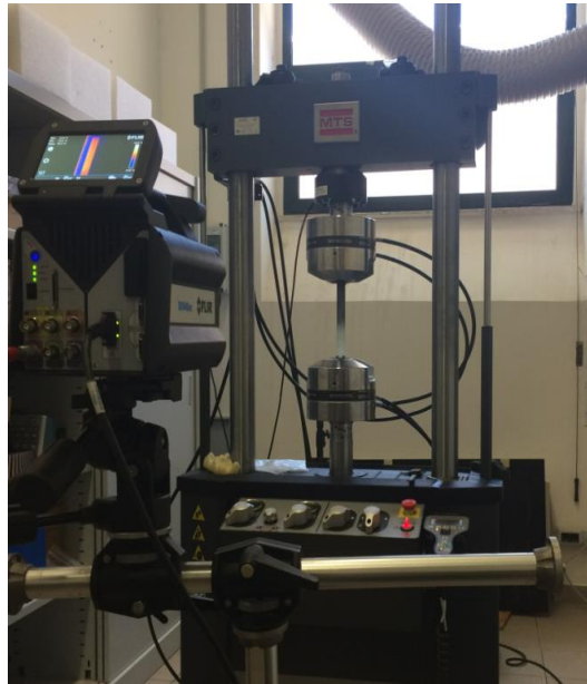
Figure1: Experimental set-up adopted for thermographic tests
