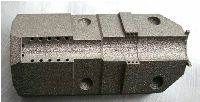
Fig. 14. Laser sintered upper component of the jig
