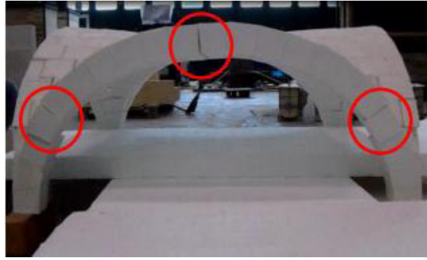
Figure 12. Horizontal (x-direction) collapse test: Arch-mechanism.
