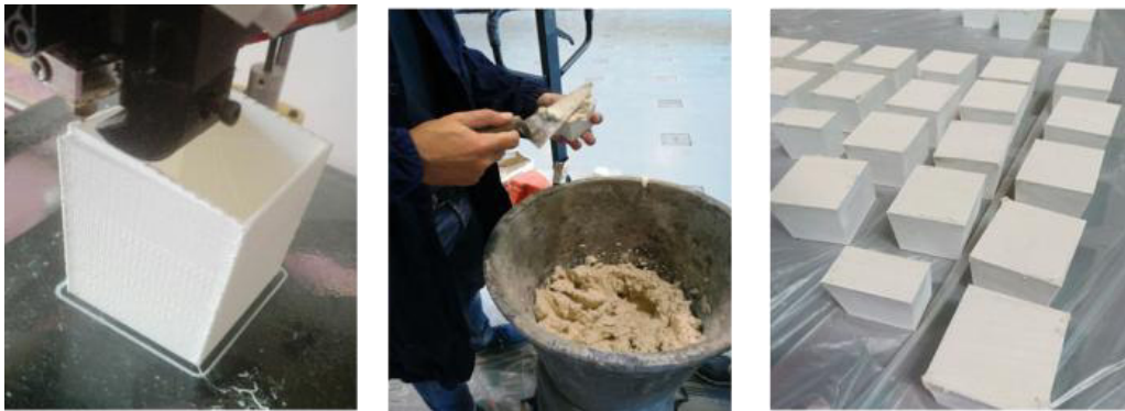
Figure 8. Manufacturing steps of the specimens' blocks.
