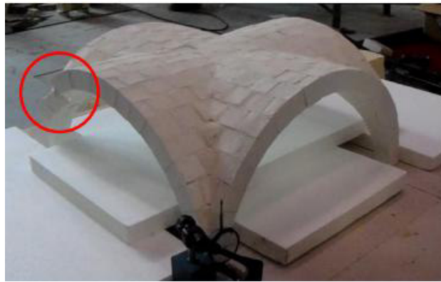
Figure 11. Vertical collapse test: Limit state before collapse.
