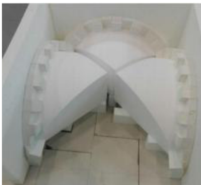
Figure 10. a) Assembly of the arch and b) disassembly of the polystyrene support.
