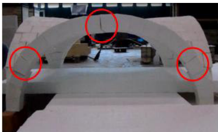
Horizontal (x-direction) collapse test: Arch-mechanism from an experimental point of view:
