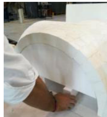
Figure 10. a) Assembly of the arch and b) disassembly of the polystyrene support.
