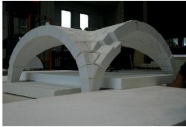
Figure 13. Horizontal (x-direction) collapse test: Limit state before collapse.
