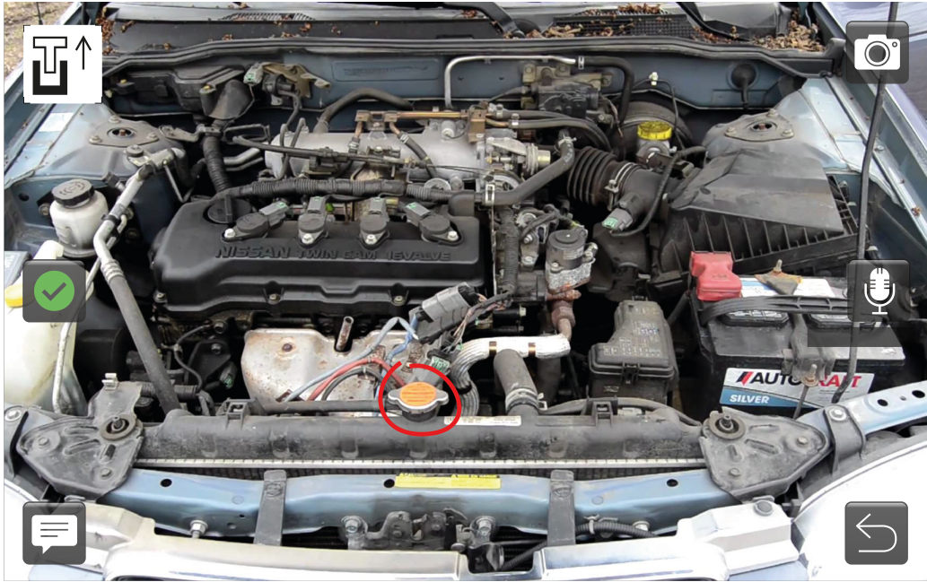
Figure 6: Application on client. The sketch drawn by the expert operator is displayed, indicating the component on which the action should be accomplished. The action is illustrated by the symbol presented on the left.
