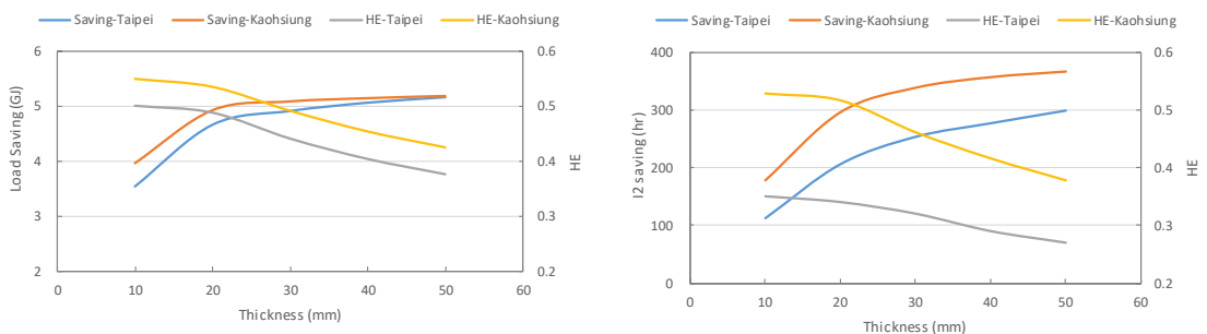
Figure 11. The energy-saving and thermal comfort efficacy of different thicknesses of PCM layers under the beneficial PCT.
