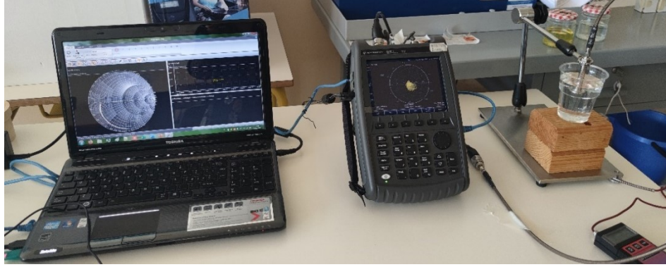
Fig. 4.1. Characterization set-up with VNA Keysight N9927A FieldFox and DAK 3.5 probe.
