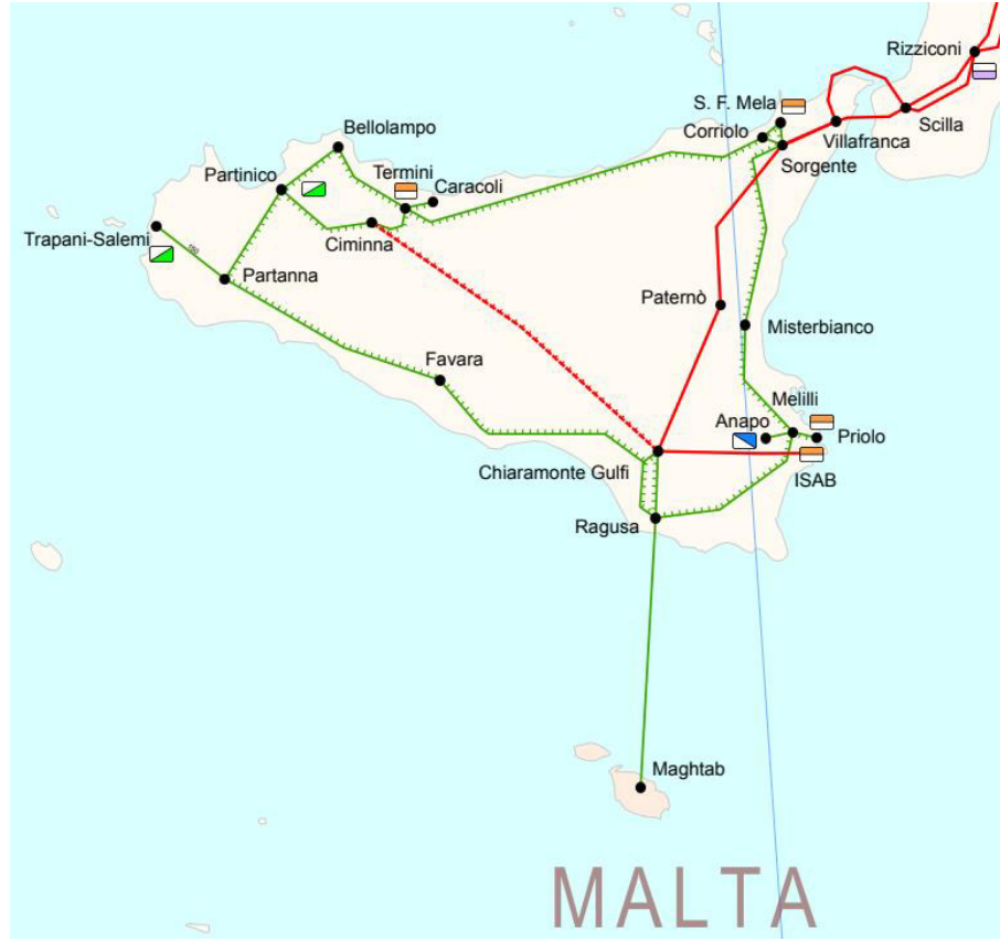
Fig. 42. ENTSO-E Sicily 400 and 230 kV transmission system representation.
