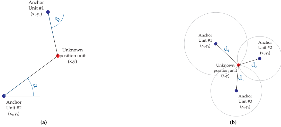
Figure 1.2: Sketch of the (a) angulation and (b) lateration position identification techniques in bidimensional space. The anchor nodes are set in the known positions (x_i, y_i) \in \mathbb{R}^2 , i = \{1, 2, 3\} while the target in the unknown position (x, y) \in \mathbb{R}^2 . The position is then determined to the angles-of-arrival \{\alpha, \beta\} and the distances d_i , respectively for the two techniques.
