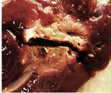
Figure 3.27 Thermal lesion in bovine liver obtained during the experimental ex-vivo validation produced using a power supply of P_{avg} = 10\text{ W} for t = 180\text{ s} . 14G MW applicator prototype [2].
