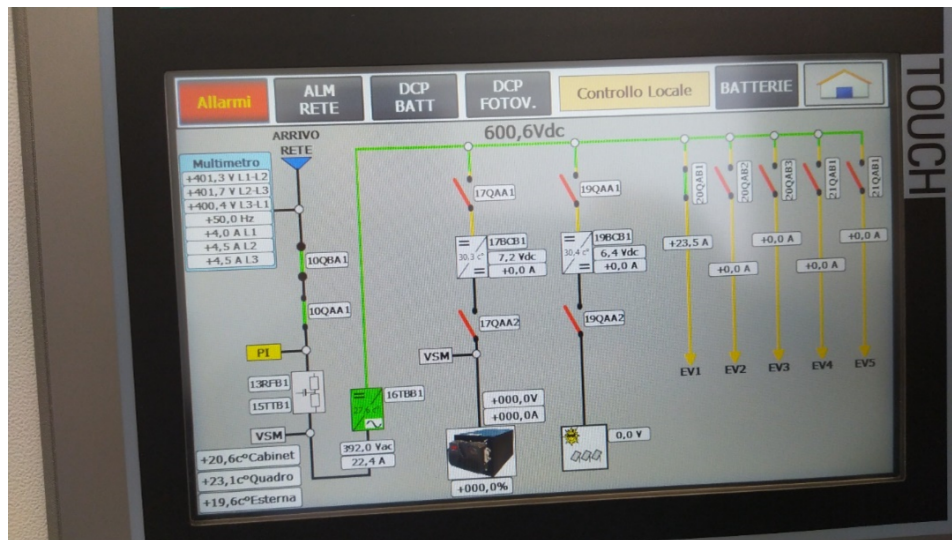
Figure 2.36: DC microgrid interface during charging test of EV1 at a V2G charging point.
