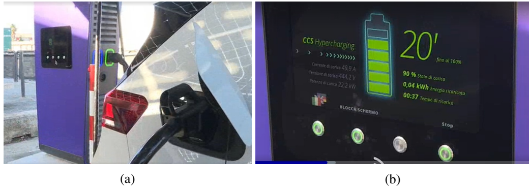
Figure 2.39: HPC fast charging station ready to operate (a) and operation panel of the station (b).
