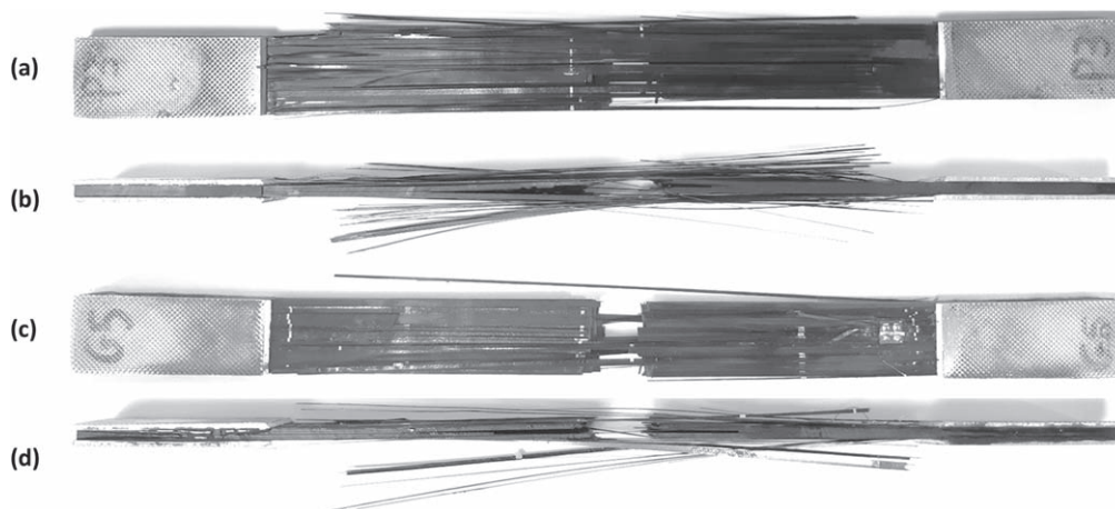
Figure 8. Tension–tension fatigue failure of specimens without BVID. Top view (a) and side view (b) of P-specimen, and top view (c) and side view (d) of G-specimen.
