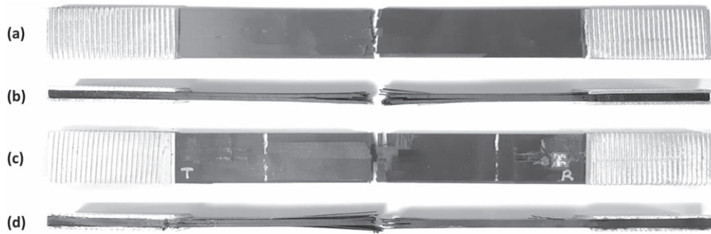
Figure 6. Tensile failure of specimens without BVID. Top view (a) and side view (b) of P-specimen, and top view (c) and side view (d) of G-specimen.
