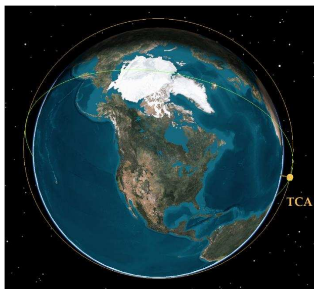
Fig. 4.9 Conjunction between Starlink 1350 (orange) and Iridium 33 fragmentation debris (green)
