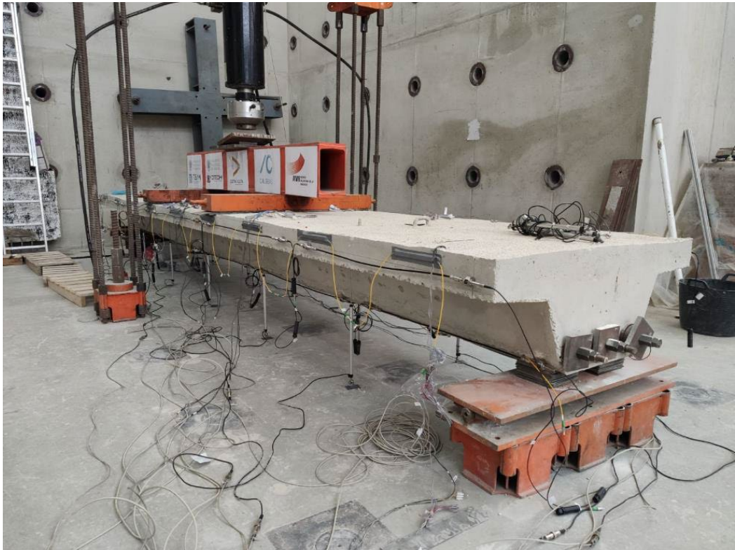
Fig. 84 - Set up of the four-point bending test.
