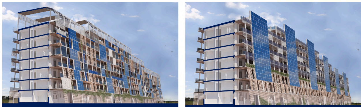
Fig. 5. Examples of possible retrofitted façade using the en-SOLEX system.
