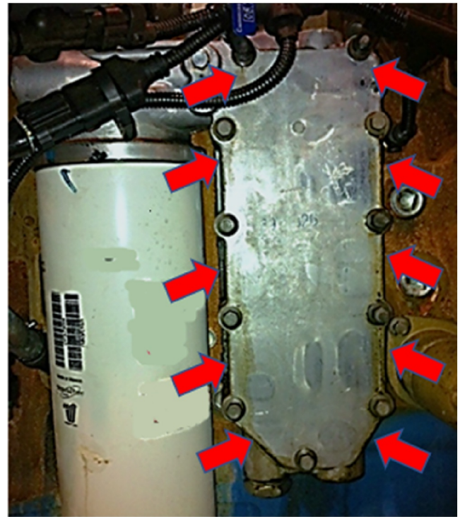
FIGURE 14 | Oil leak through screw holes.
