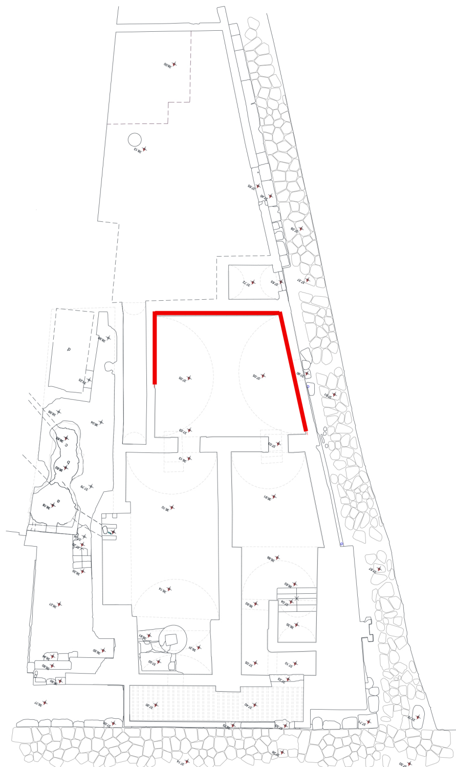
Figure 3. Plan of Women's Thermal Baths, with the radiant walls highlighted (red lines).
