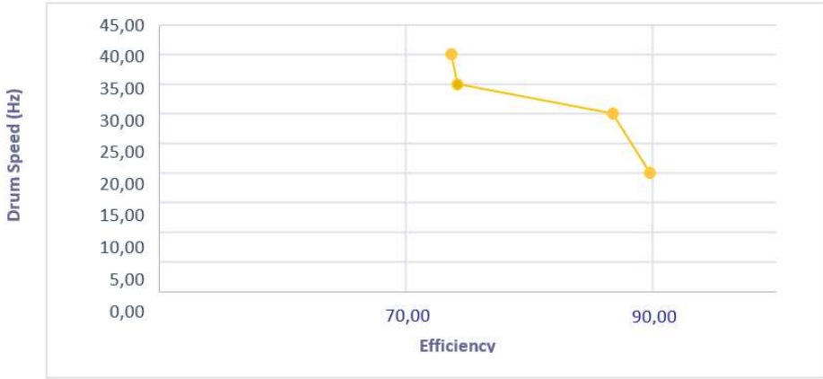
Figure 52- Variation of the separation efficiency with the drum speed
