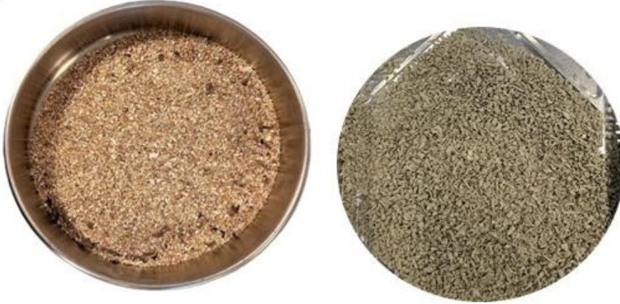
Figure 18- Mix 1, Sand and PP plastic
