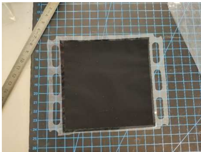
FIGURE 3. Structure constituted of CCM and sub-gasket after the cutting process. The apertures guarantees the stream of reactants and products within the PEMFC stack.
