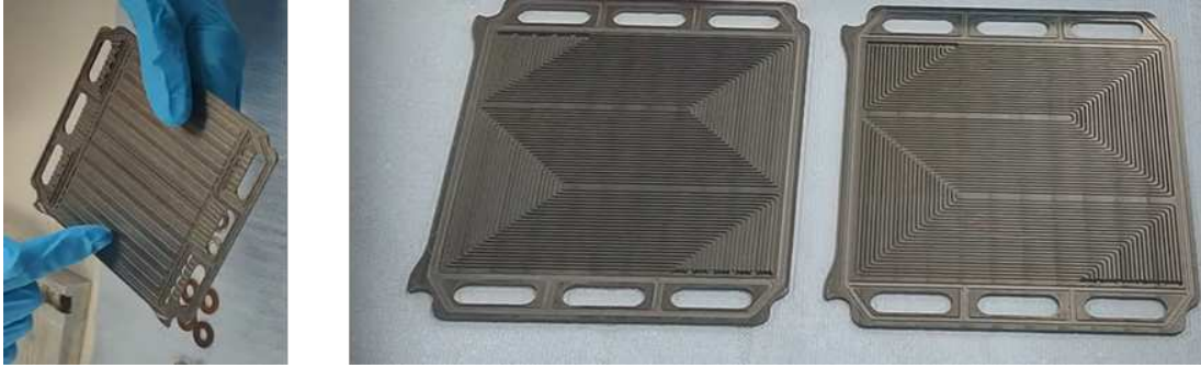
FIGURE 2. Cathode coolant flow field (left), cathode and anode reactants flow fields (right).
