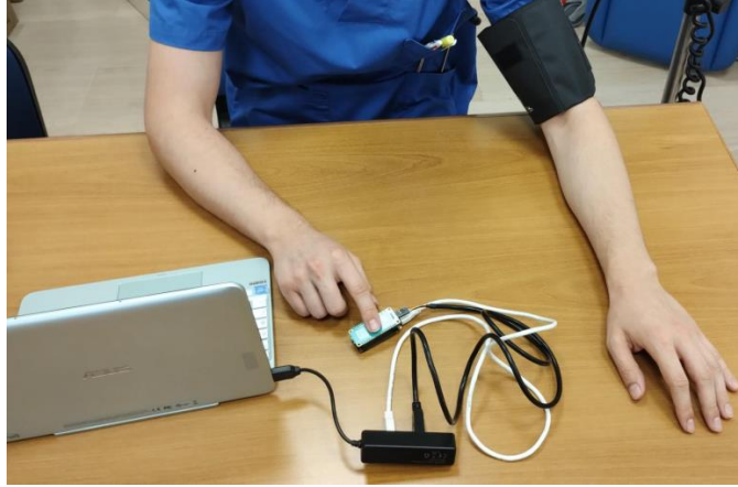
Figure 3.7. Experimental set-up for blood pressure data acquisitions: PPG signals were acquired by positioning the right index finger on the PPG sensors and SBP and DBP via sphygmomanometer.
