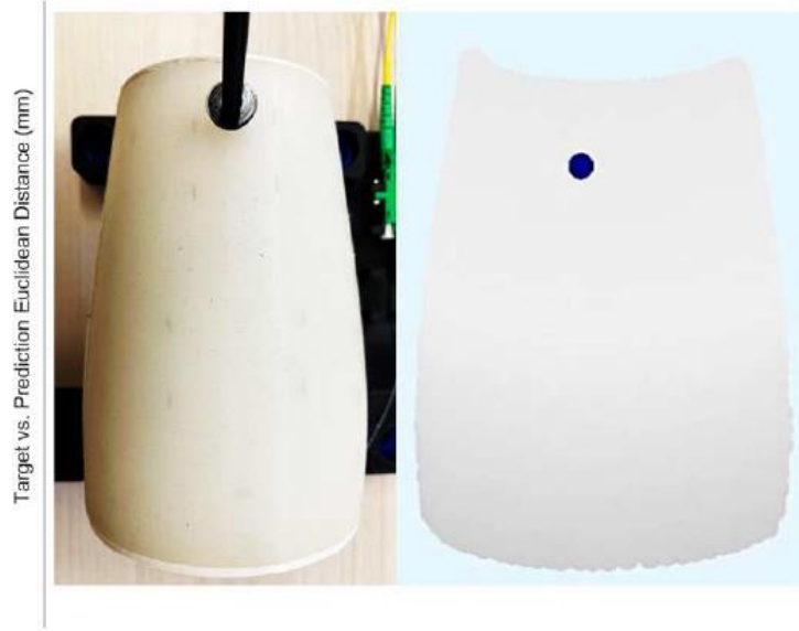
Figure 4.5. Example of real-time localization of a touch event by the on-the-edge AI algorithm deployed on the MCU.
