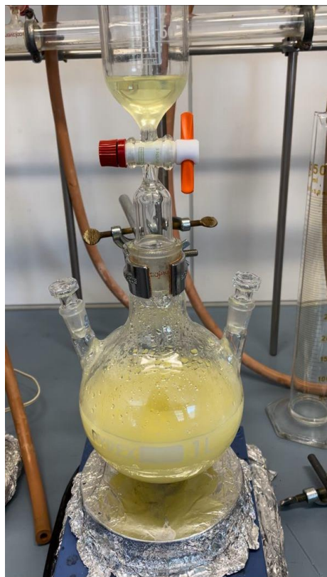
Fig. 6.1 - Photograph of the reaction apparatus used for the cellulose oxidation during the dropwise \text{NaClO} addition.
