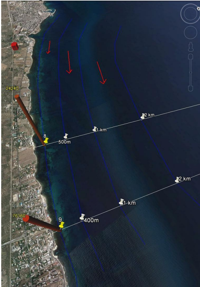
Fig. 6. Transects monitoring: O.V. cell concentration in columns, water current flow (red), bathymetric lines (blue), transects (white), current fortnightly monitored spots (yellow), ideal additional spots (white).
