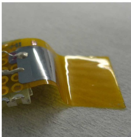
Fig. 3 Flag prototype tested in the wind tunnel; the residual stress of the polycrystalline layers on Kapton generates a bending of the Kapton foil.
