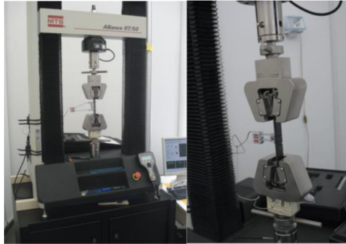
Figure 6. Setup of tensile test and detail of a joint under test
