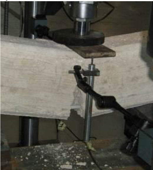
Fig. 10. Detail of the different behaviors; a) specimen reinforced with PET bars; b) specimen reinforced with CFRP strips.
